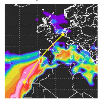
QSO. During the QSO, I received 5 reflections from Fernando, 3 pings (160ms/6dB, 120ms/2dB and 120ms/6dB) and 2 bursts (340ms/6dB and 4sec/7dB). What has been decoded from the longest reflection is shown on the WSJT screenshot.
