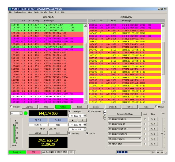
Ricardo is using 80W and 2×9 elements antennas. I'm using 1,2 kW and 2×9 elements too. It makes a difference of more than 10 dB, which is somehow reflected in the reports seen. I saw Ricardo -19 dB at best and he saw me -11 at best. At -11 dB, my signal was barely audible in a reduced bandwidth. Hence, even in CW, a QSO would have been hard to achieve (at same RF power level both sides).
