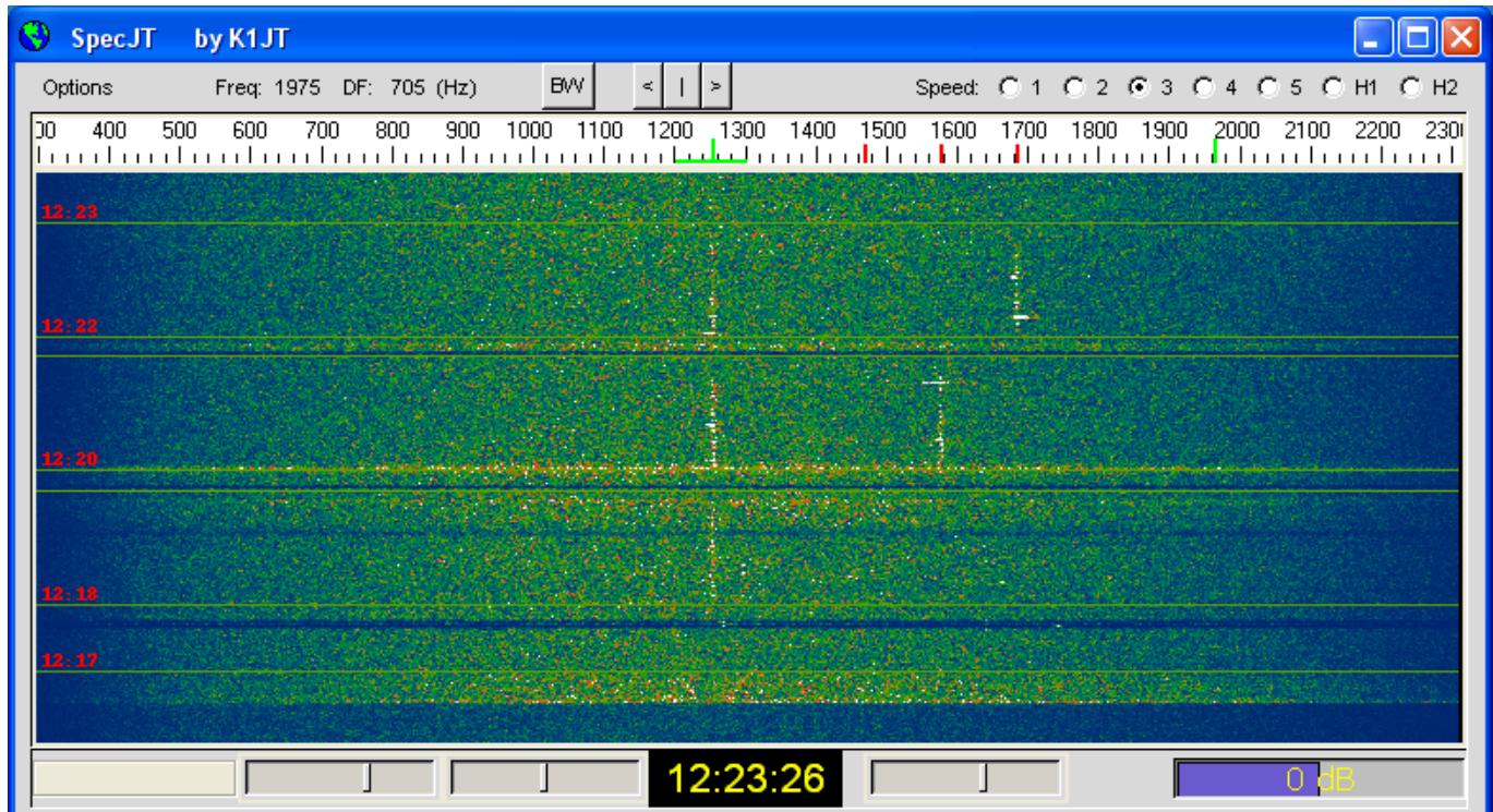
Test avec OH4LA / Test with OH4LA (best received -18 dBJT / best I was received -17 dBJT : 123100 0 -17 -0.5 -151 9 # OH4LA ON4KKG J010 000 1 10)
