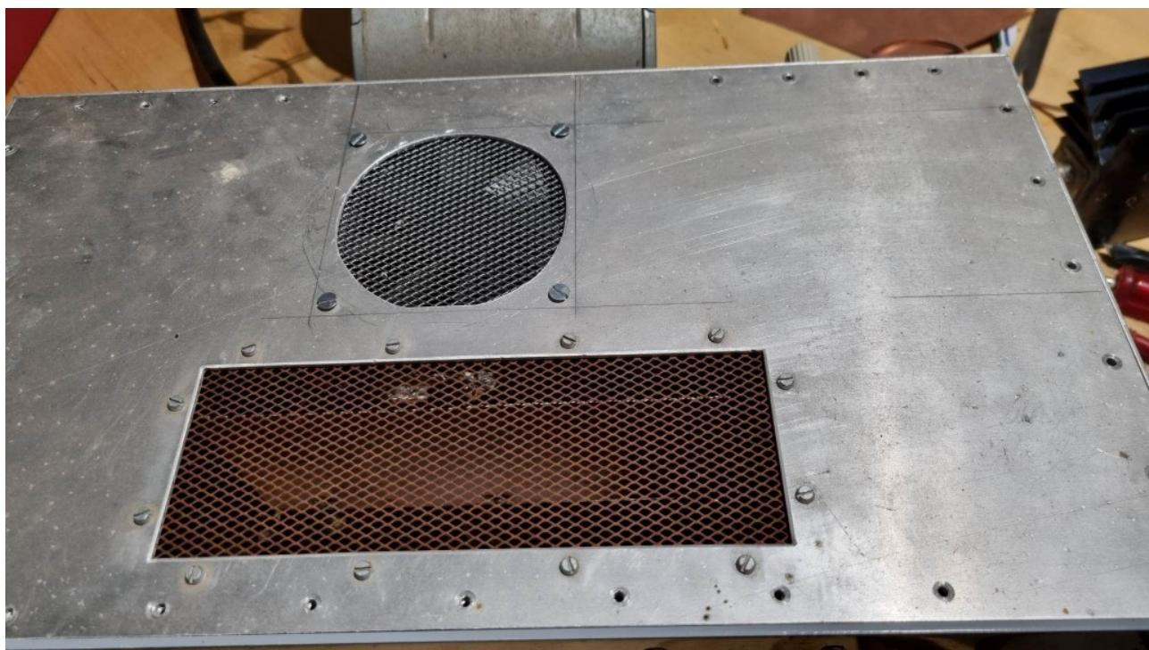
Since I'm active on 144 MHz in EME (earth-moon-earth), I need RF power. After a 300W, then a 600W version, I built a 1kW+ SSPA (Solid State PA) in 2017 (a video relating to this amp is available [here](#)). It's based on a kit from Jim, W6PQL (very reliable equipment). The transistor used is a BLF188XR. This amp worked perfectly until mid-June 2023. During a digital transmission on a hot day (31°C), it stopped
