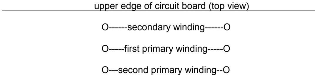
Transformers T2 and T3 in the 20m/30m kit are wound on BN-61-2402 cores. These two cores are in a separate poly bag within the cores and wire sub-kit bag. Please note the marking BN-61 to identify the two cores. RFC1 in the 20m/30m RXTXv6.2 kit is wound on a BN-43-2402 core that is not specifically identified in the cores and wire sub-kit bag. These two core types have different AL values and high frequency loss and should not be used for the wrong application in the kit.
