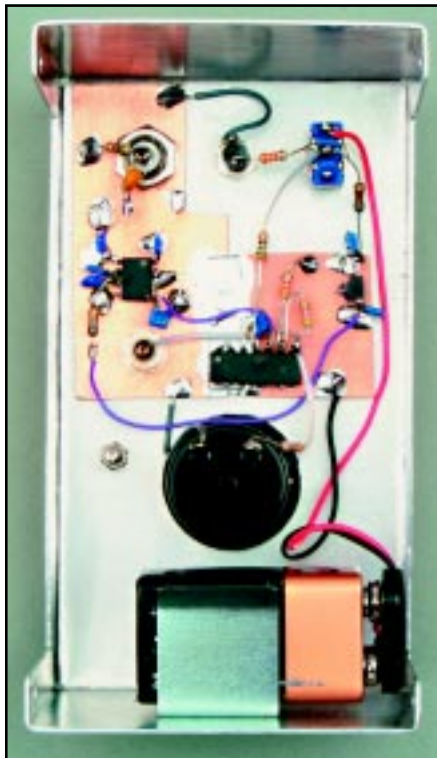
An inside view of the wattmeter showing its "dead-bug" construction and simplicity.
