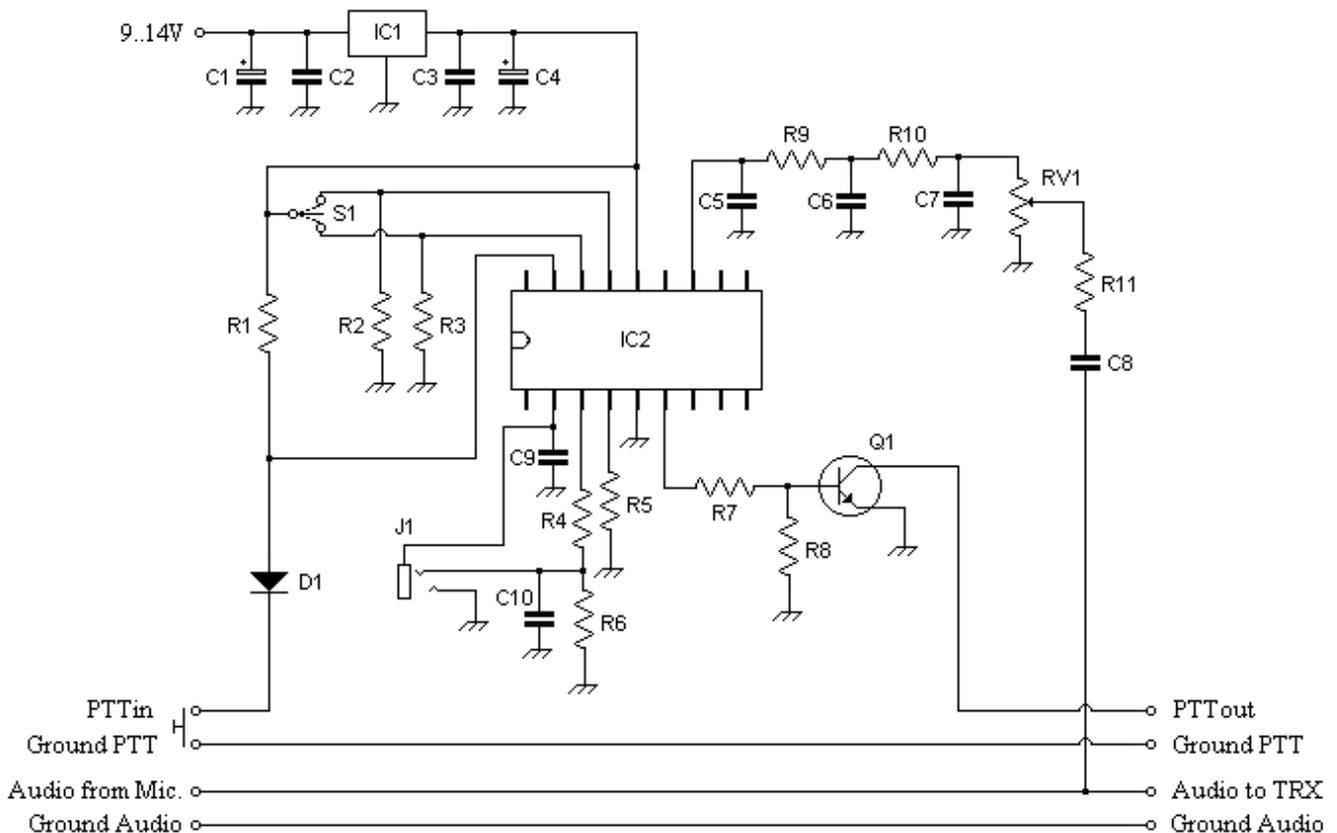
The switch S1 allows to select one of the three operating modes.
